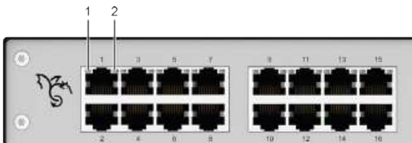
Fig. 48 Front side - LEDs at I/O Ports, 1G Cat X
