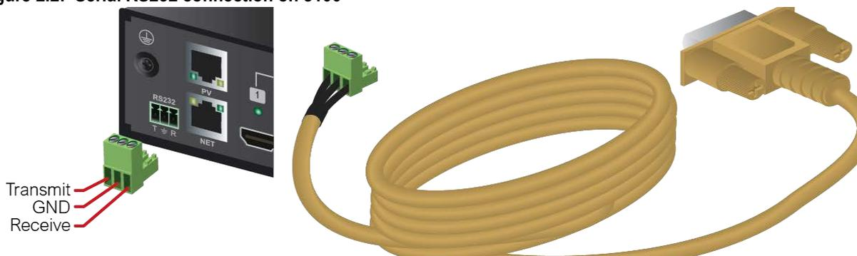
**Table 2.1: RS232 (DB9F/3P) cable pinout**
