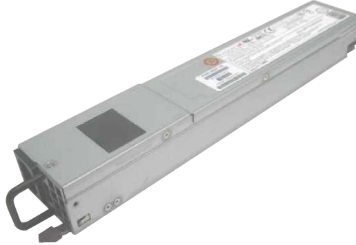
Figure 4.15: Express Fabric Chassis Power Supplies
