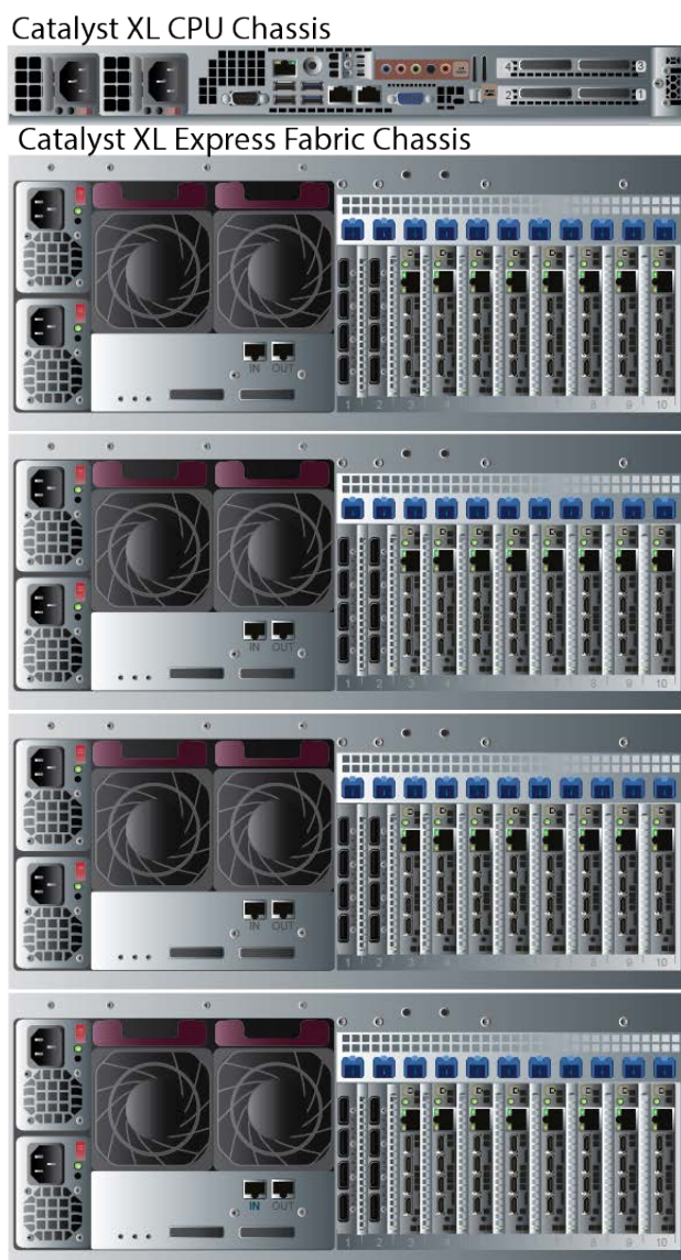
Figure 1.2: One CPU Chassis Control up to Four Express Fabric Chassis
