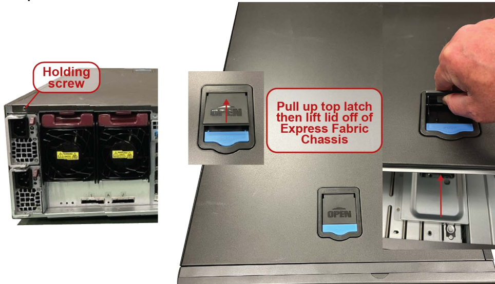
Figure 6.10: Express Fabric chassis cover removal
