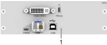
Fig. 26 Interface side - USB/Video Connection Status LED L474-BSHxV
