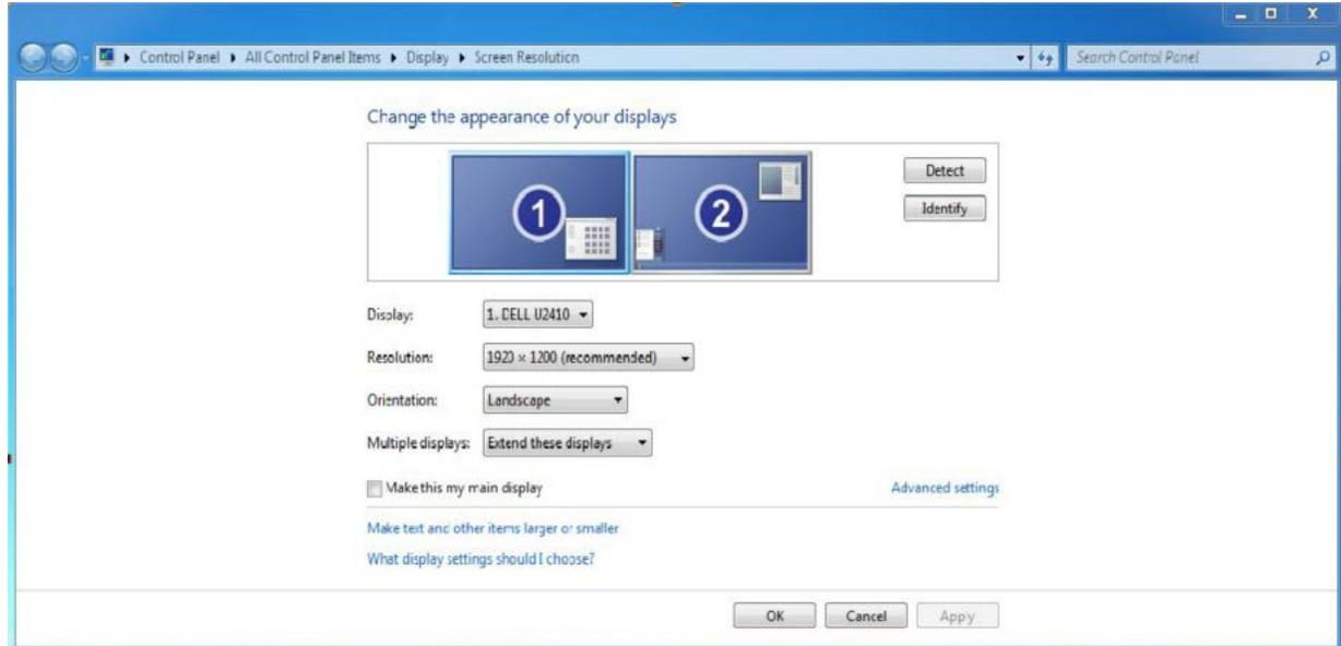
**Note:** The screen may go black if the wrong resolution is chosen. The CRS-5K will revert to the last working resolution in a short while.
