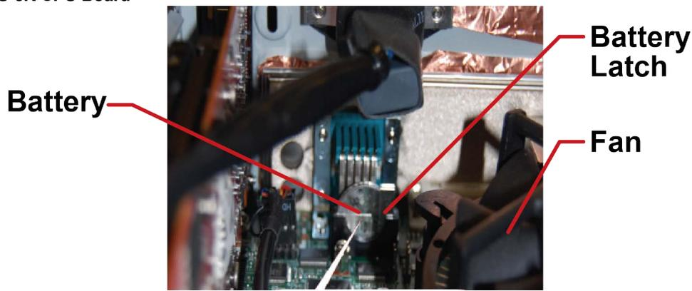
**Caution:** Removing the battery will erase key information such as the date, boot order, and RAID settings. Write down the current values for these settings before removing the battery.
