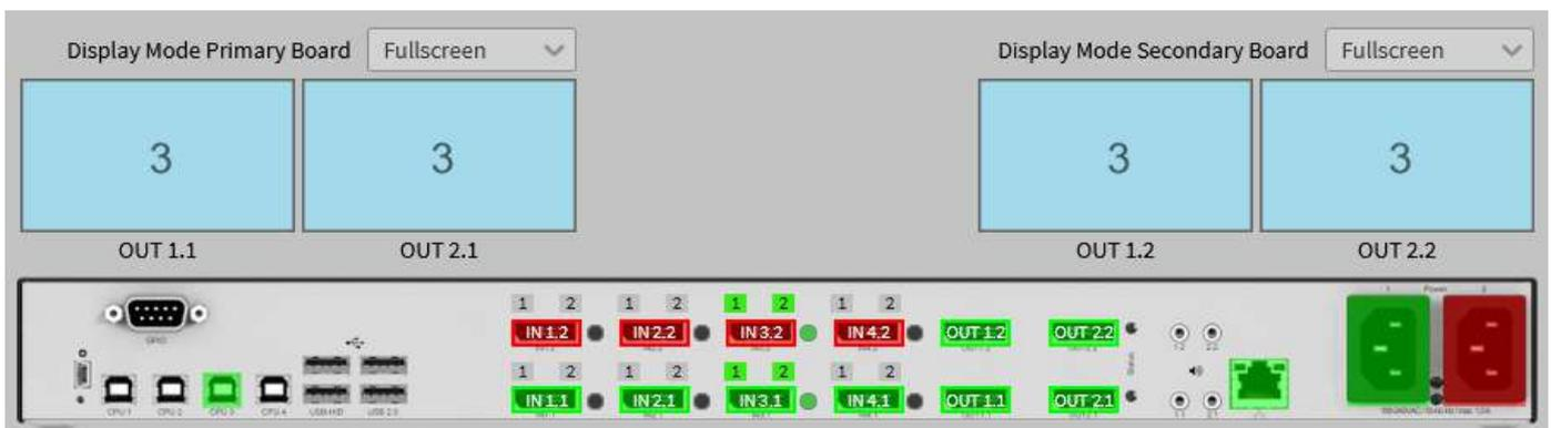
Fig. 166 Web UI menu **Device Status** - Synchronous focus on one input in mirrored Fullscreen Mode (2)
