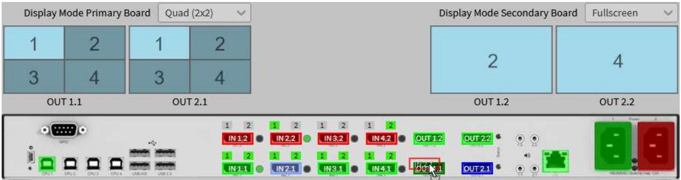
Fig. 178 Example - Focusing on another input and changing the display mode by dragging
