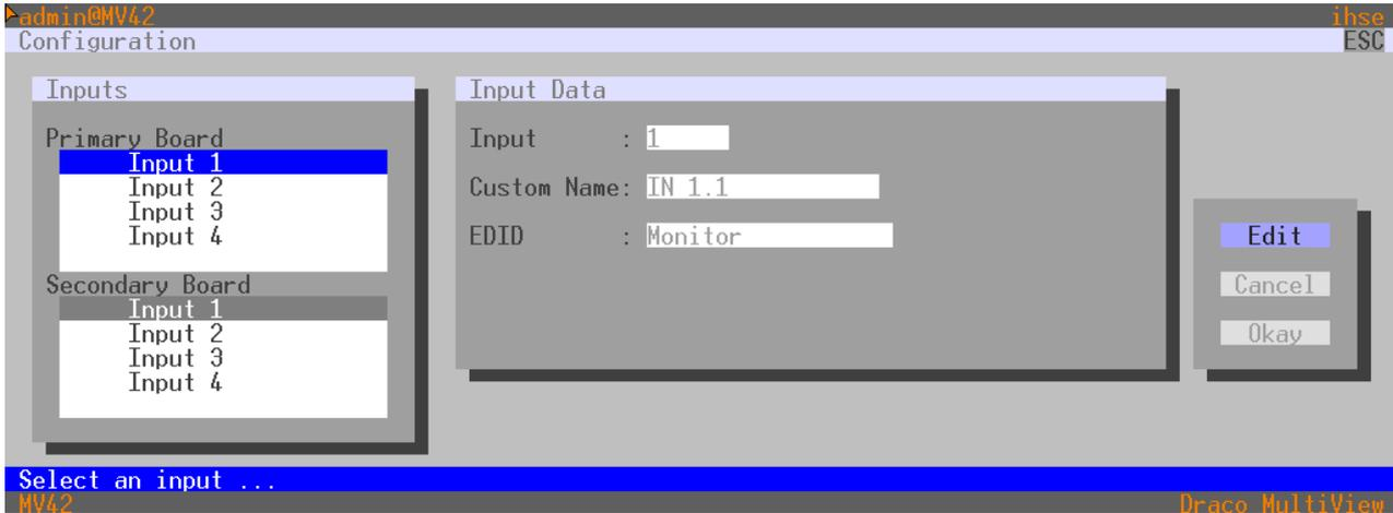
Fig. 62 OSD Menu **Configuration - Inputs** (example with dual-head device)
