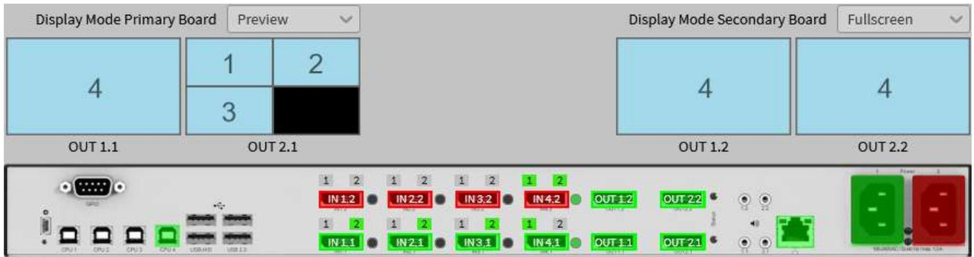
Fig. 177 Web UI menu **Device Status** -Asynchronous change to another display mode (2)
