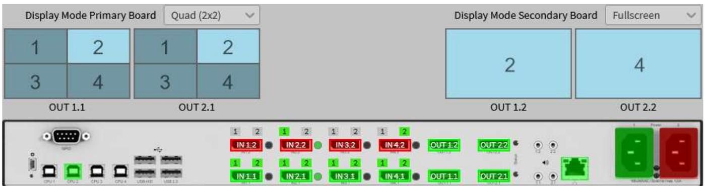
Fig. 175 Web UI menu **Device Status** - Asynchronous focus on another input in Quad Mode (2)
