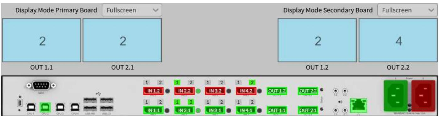
Fig. 180 Example - Changed display mode by focusing on another input by dragging
