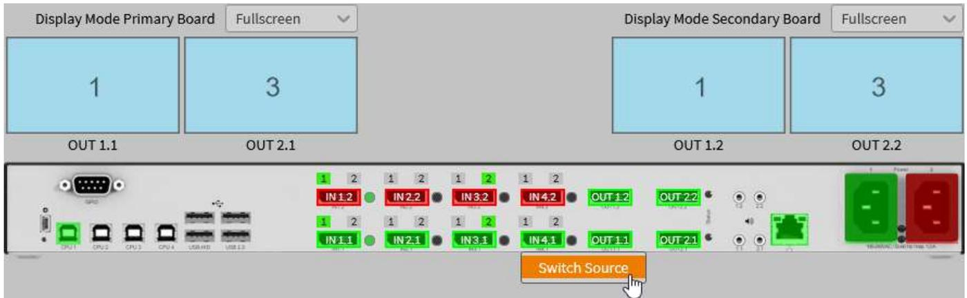
Fig. 167 Web UI menu **Device Status** - Synchronous focus on one input to mirrored Fullscreen Mode (1)
