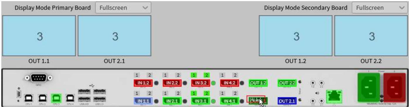
Fig. 169 Web UI menu **Device Status** - Synchronous focus on two inputs in individual Fullscreen Mode (1)
